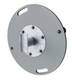
The bearing house is made from hot dip galvanised steel. The bearing shaft is made from stainless steel AISI304. The bearing itself is made from Polyoxymethylene (POM), an engineering thermoplastic with a high stiffness, low friction, and excellent dimensional stability.
