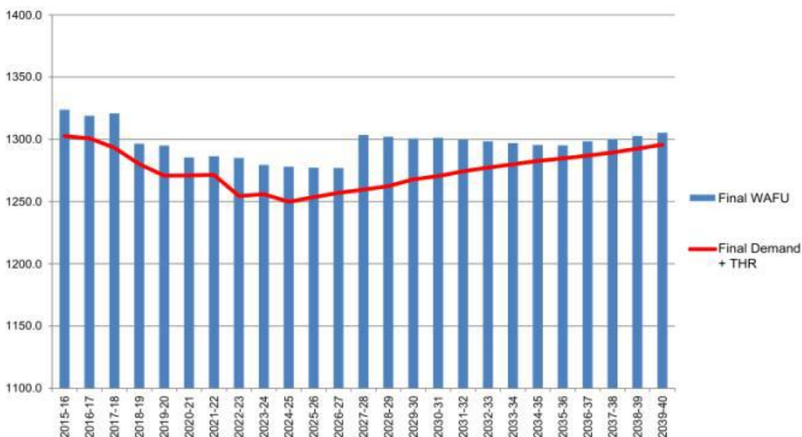
Figure 4-6: Supply/demand balance with the AWS preferred plan implemented showing the water available or use (WAFU) and final demand plus target headroom (THR) 18
