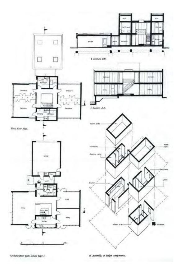
Figure 13: House Plan showing the combining of the various component parts
